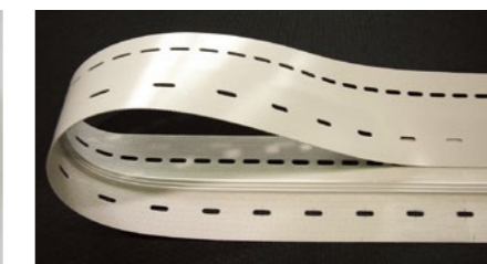
Holes punched through the belt are used in suction conveyance.
