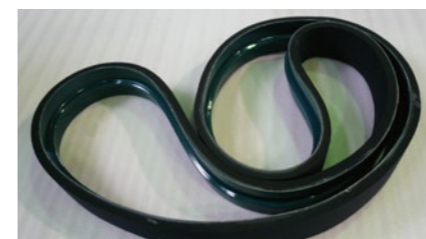
Sponge on the belt surface and V-guides on the belt backside are used in sandwich conveyance.
