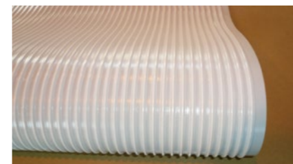
Multi-row V-guides on the belt surface are used to align granular transport.
