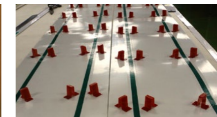
Marking and cleats are used to position the materials being conveyed.
