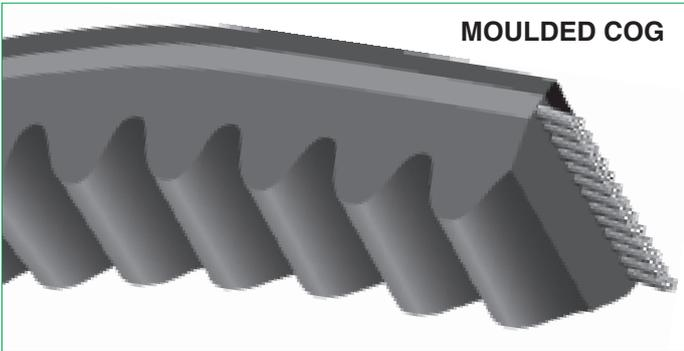
**TORQUE-FLEX® - Narrow "XP"** high performance belts are manufactured in accordance with European standards **ISO 4184**, **DIN 7753** and are approved by **API** (American Petroleum Institute). The belt structure guarantees high transmittable power while the moulded cog profile provides higher flexibility with small diameters pulleys.
